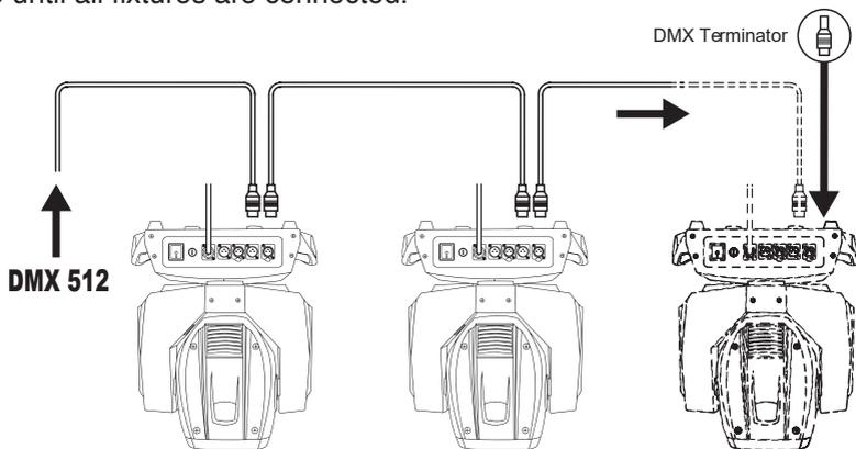
**A word on termination:** DMX is a resilient communication protocol, however errors still occasionally occur. Termination reduces signal errors, and there-
