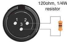
To build your own DMX Terminator: Obtain a 120-ohm, 1/4-watt resistor, and wire it between pins 2&3 of the last fixture. They are also readily available from specialty retailers.
